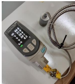
Gambar 14. Pull off test
