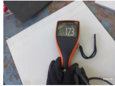
Gambar 12. Tahap Pengujian Dry Film Thickness (DFT)
