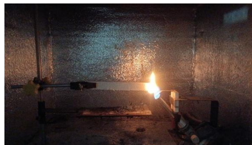
Figure 7. Horizontal burning test procedure.
