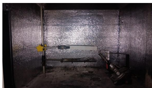
Figure 2. Horizontal burning test setup
