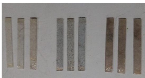
Figure 6. Horizontal burning test spesiment.
