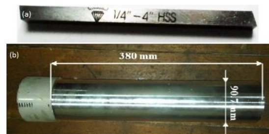
Gambar 1. (a). Pahat potong bubut HSS, (b) Material paduan magnesium
