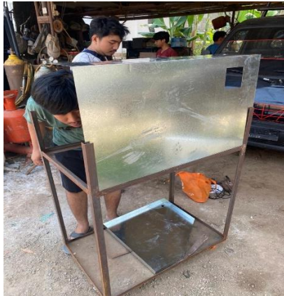
Gambar 8. Alat kabin Sandblasting
