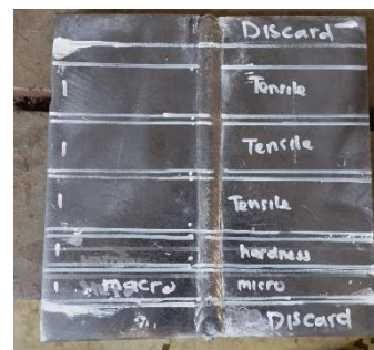
Gambar 1. Cutting Plan Hasil Pengelasan
