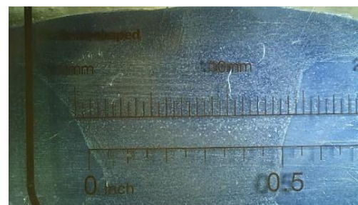
Gambar 4. Weld Zone 1 Kali Repair
