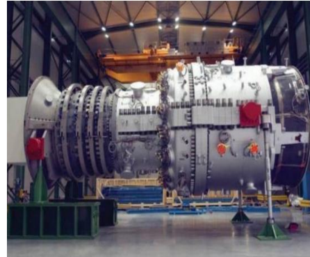
Gambar 6 Turbin Gas Heavy Duty (Sumber: PT.SumberdayaSewatama, 2013)
