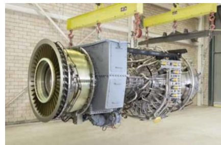
Gambar 7 Turbin Gas Aero-derivative (Sumber: PT.SumberdayaSewatama, 2013)
