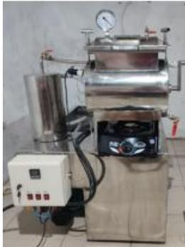
Gambar 1. Mesin Vacuum Frying
