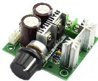
Gambar 17. PWM ( Pulse Width Modulation )
