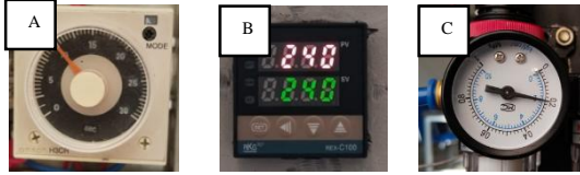
Gambar 5. A. Timer, B. Temperature controller, C. Air Regulator
