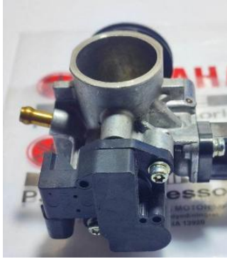
sumber: 6 https://zd-img-global.slatic.net/g/p/d31059bc07d69bcd6c0b4fddfc8015e2.jpg_720x720q80.jpg Gambar 6 Throttle Body 28 mm
