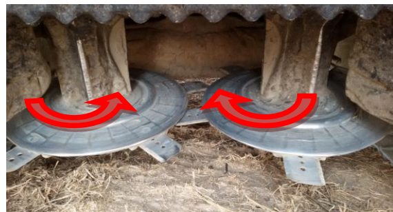
Gambar 2. Arah putaran disc holder Slicer Sugarcane Harvester saat proses pemotongan batang tebu saling berlawanan arah jarum jam
